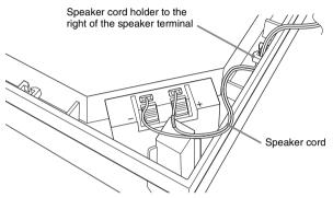
**2** Thread the speaker cord through the gap along the side of the subwoofer.
