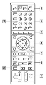
Number 5, ODD, ∠ +, and ► buttons have a tactile dot. Use the tactile dot as a reference when operating the remote.
