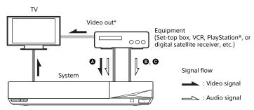
\* This connection is unnecessary for connection (A) (HDMI connection).
