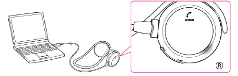
Charging starts when the headset and the computer are connected. Make sure that the indicator (red) lights up. Charging is completed in about
