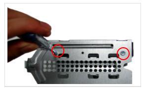
**Step 5.** Using the enclosed magnetic screwdriver, remove the two (2) indicated screws and set aside.
