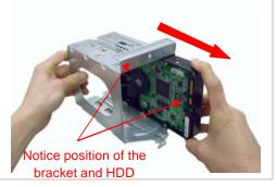
**Step 7.** Pull out the original hard drive from the bracket in the direction of the arrow. **IMPORTANT!** Take note of the original position of the drive inside the bracket.
