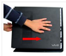
**Step 14.** Re-assemble the chassis panel cover. And reinstall the screws removed in step 1. Connect your PC and continue with the recovery following the instructions on the back of the recovery disk's case. Return the original hard drive to Sony following the included shipping instructions.
