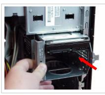
**Step 10.** Slide the hard drive bracket enclosures back inside the unit, making sure all holes are lined up.
