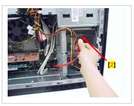
**Step 13.** Gently reconnect the serial ATA cable [2] into the hard drive as indicated above.
