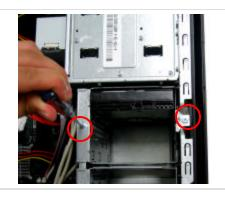
**Step 11.** Using the enclosed magnetic screwdriver, reinstall the two (2) previously removed screws. **IMPORTANT!** Do not over tighten the screws.
