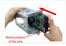
**Step 8.** Gently insert the new hard drive into the bracket in the direction of the arrow. Align the new drive in the same position as the original hard drive.
