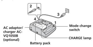
**1** Set the mode change switch of the AC adaptor/ charger to CHARGE.
