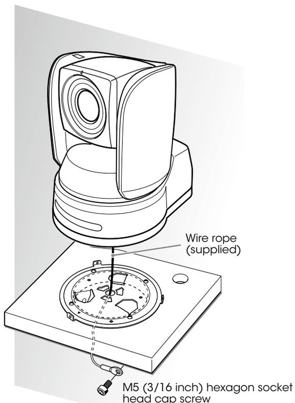
**6** Insert the protrusions on the ceiling bracket (A) into the spaces prepared in the ceiling bracket (B) with the a hole in the front of the ceiling bracket (A) aligned with the hole on the ceiling bracket (B), and temporarily attach them by turning the ceiling bracket (A) with the camera counterclockwise.
