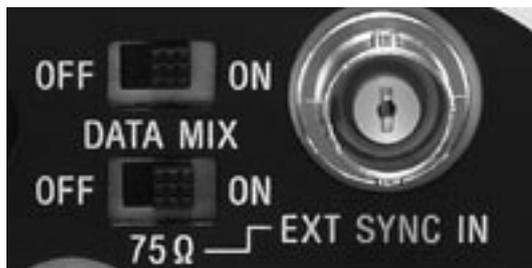
DATA MIX switch on the BRC-Z330 (rear)
