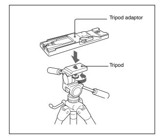
**2** Place the camera on the tripod adaptor, and slide forward it along the groove of the tripod adaptor until it clicks.
