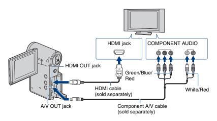
• You cannot connect the HDMI cable and the component A/V cable at the same time.
