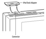
To remove the iPod Dock Adapter, pull it up with your fingernail or a flat object using the slot inside the adapter.
