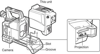
2 Slide the unit along the groove on the camera, and press firmly until fixed.
