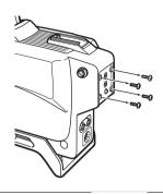
Attach the battery adaptor mounting bracket (Part number 3-690-850-01; not supplied) with the screws removed in step 1.
