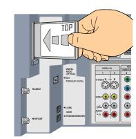
Inserting the CableCARD incorrectly may result in permanent damage to the card and the TV.
