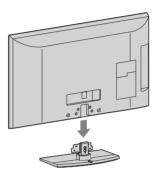
**2** Use the supplied screws to attach the TV unit to the Table-Top Stand.
