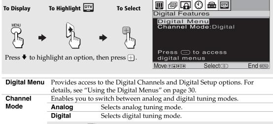
Press the button on the remote control to directly switch to analog or digital Channel Mode.
