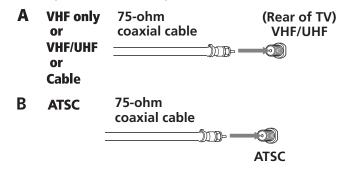
Use option A to connect the TV to a cable system or an antenna with a 75-ohm cable.
