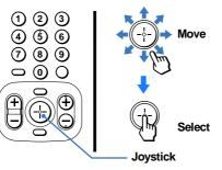
The supplied remote control has a joystick which moves the on-screen selector in eight directions. In most cases, moving the joystick up, down, left or right will cause the selector to move in the selected direction.
