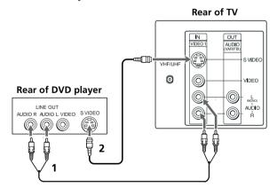
For optimum picture quality, use S VIDEO instead of the yellow A/V cable. S VIDEO does not provide sound, the audio cables must still be connected.
