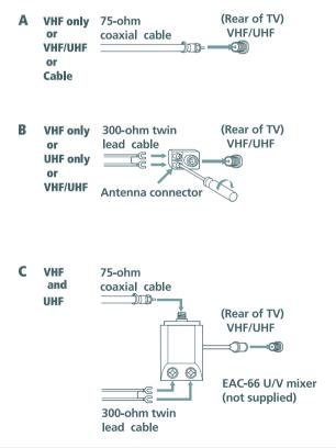
A If you are connecting to an indoor or outdoor antenna, you may need to adjust the orientation of the antenna for best reception.
