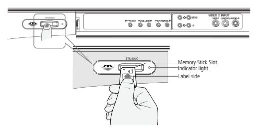
🖾 Be sure to insert the Memory Stick in the correct direction. If the Memory Stick is forced in the wrong way, it may become damaged.
