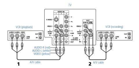
To perform tape editing, set the TV to the video input intended for playback by pressing the TV/VIDEO button on the remote control.
