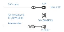
Select CABLE or antenna (ANT) mode by pressing ANT on the remote control.
