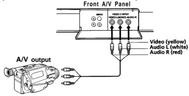
If you have an S VIDEO equipped camcorder, you can use an S VIDEO cable for optimum picture quality.
