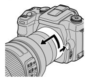
2 Hold down the lens release on the teleconverter and turn the lens counterclockwise until it stops. Carefully lift the lens out of the teleconverter mount.
