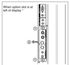
The location of the option slot differs according to the model. On models with multiple option slots, use a slot that supports video/communication functions (VIDEO/COM port). Consult the documentation of the FWD series product for more information.
