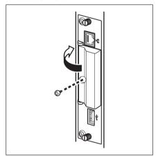
**2** Open the memory card slot cover and insert the CF card into the memory card slot.
