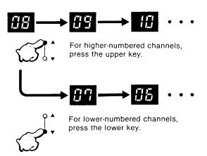
This TV tuner is preset at the factory to receive VHF channels 2 through 13 with the CHANNEL keys. To add UHF or CATV channels or to erase inactive channels, see page 14.
