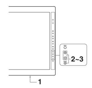
**1** Turn on the unit with the  $\odot/\dot{\bigcirc}$  (power) switch on the bottom panel.
