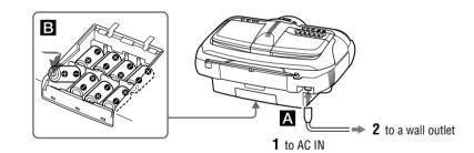
Connect the AC power cord A or insert eight R20 (size D) batteries (not supplied) into the battery compartment B.
