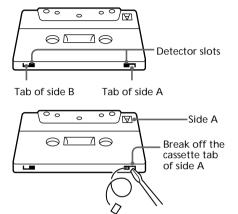
If you later want to reuse the tape for recording, cover the broken tab with adhesive tape. However, be careful not to cover the detector slots which allow the tape player to automatically detect the type of tape.
