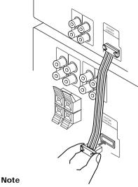
The system cable is used for exchanging signals between the tape deck and the CMT-SD1/SD3 (or MDS-SD1). If you do not connect the cord firmly, the tape deck may not operate correctly.
