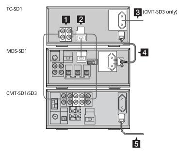
1 Firmly connect the system cable to the SYSTEM CONTROL jack on the CMT-SD1/SD3.
