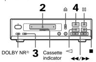
2) This tape deck is equipped with the Dolby B-type noise reduction system.
