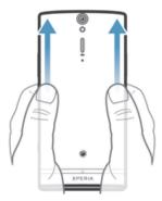
• Using your thumbs, press down on the back cover, then slide it upwards.
