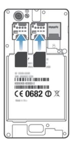
Remove the battery cover, then insert the SIM card into its slot with the goldcoloured contacts facing down.
