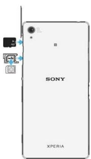
! Make sure you insert the nano SIM card into the nano SIM card holder before inserting it into the device. Also, don't confuse the nano SIM card slot with the memory card slot.
