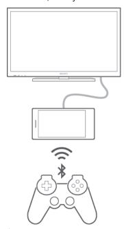
To set up a connection between a DUALSHOCK™3 wireless controller and your device, a USB On-The-Go adapter is required.
