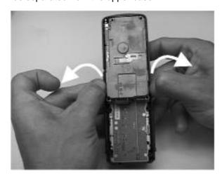
5. The electronical part (= MMI board with RF/logic unit as a whole) is held onto the upper case by a claw on either side. Therefore, in order to release the upper case from the electronical part, squeeze both sides of the upper case gently to the outside and at the same time push the electronical part upward.
