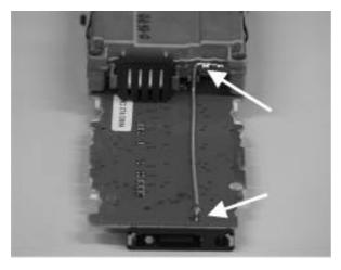
9. When unsoldering or resoldering the coax cable, be very precise and use the exact correct amount of soldering, not too much, not too little. The RF level towards the car connector can be affected drastically by bad solderings.
