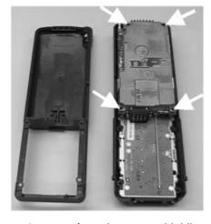
4. Remove 4 screws from the upper shielding.
