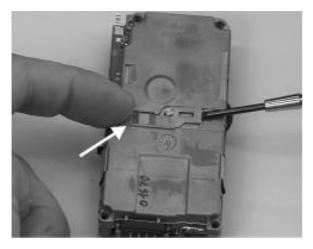
7. To separate the RF/Logic block from the MMI board, lift the spring slightly using a small flat screwdriver while pushing it to the right with your finger.
