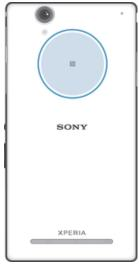
The location of the NFC detection area is not the same on all devices. When sharing data with another device using NFC, refer to the User guide of the other device for more information.
