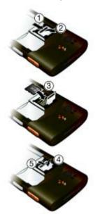
Open the cover and insert the memory card with the gold-coloured contacts facing down.
