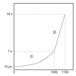
When Auto Shutter is selected, the exposure time is adjusted automatically, based on the brightness of the subject. At this time, the reference level (target point) is set in the AutoExposure register.
