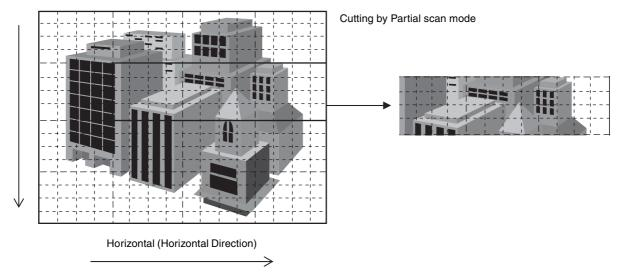
The minimum unit size for partial scan is  $32 \text{ pixels} \times 24 \text{ lines}$ . The cut-out position can be set in unit of 4 pixels  $\times 4 \text{ lines}$ . For high-speed scanning, set the maximum packet size.
