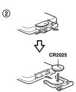
**3** Insert the battery compartment back into the unit and secure it with the screw. (See Fig. A-3)
