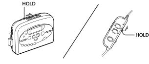
Set the HOLD switch to the direction of the arrow to lock the controls.
