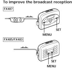
• For FM: Extend the cord of the remote control, the aerial (FX487 only). Extend the headphones/earphones cord, the aerial (FX485/FX483 only). If the reception is still not good, press MENU repeatedly to set the cursor to FM MODE or FM SENS in the display. Then press SET to choose the mode for best reception.
