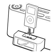
Adjust the rear support forward or backward checking the back of the iPod fits snugly against the rear support to protect the connector
