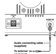
2 Press AUDIO IN to display "AUDIO IN". **3** Play the equipment connected to the
