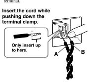
**4** Make sure the AM loop antenna is connected firmly by pulling softly.
