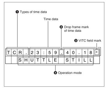
When basic menu item 005 of the setup menu DISPLAY INFORMATION SELECT is set as anything other than OFF, the video signal output from the COMPOSITE (SUPER) output connector, SDI (SUPER) output connector (for J-10SDI/30SDI only) or DV connector contains superimposed character information (overlaid display), including time code, menu settings, or alarm messages.
