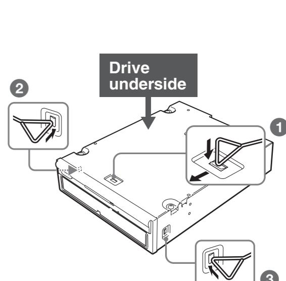
**GB** Use the ejection pin to press the three panel pins, releasing the pins.
