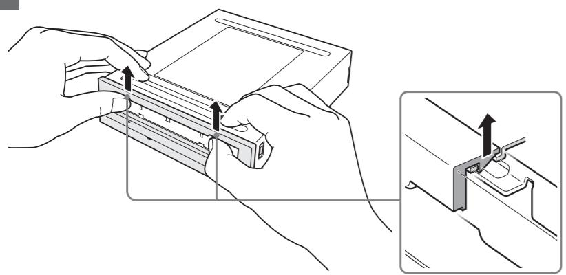
**GB** Push up the panel as illustrated, releasing the pins, and then remove the front panel.
