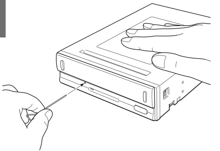
**GB** Insert the ejection pin into the emergency eject hole.
