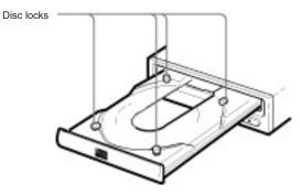
**4** Gently push the tray or press the eject button to close the tray. The drive will begin reading the Table of Contents (TOC) data when it accepts the disc. The busy indicator lights up in amber while the drive is reading the TOC.
