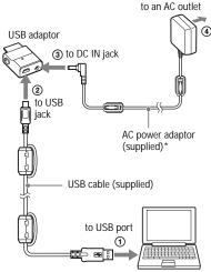
\* When transferring audio data, make sure to connect the AC power adaptor to the USB adaptor. You cannot transfer audio data if they are not connected.
