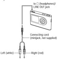
MiniDisc recorder, AV amplifier, active speaker, cassette recorder, etc.
