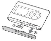
4 Slide the side part (1) and remove the two screws (2) on the side of this player.
