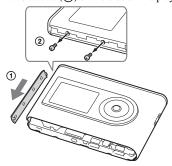
5 Push the bottom into the player with your finger and pull out the inside of the player in the direction of the arrow below.
