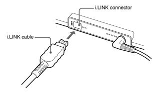
4 Connect the other end of the supplied i.LINK cable to the i.LINK connector of the port replicator on the personal computer.
