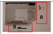
**Step 14.** Position the new ODD (Label side down) and identify the correct bracket with the correct side to be secured. Notice the different shape of each bracket and the alignment of the Bracket and ODD screw holes.
