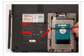
**Step 7.** Insert the enclosed screwdriver in the notch exposing the ODD Bracket (metal). Push to remove the ODD.
