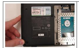
**Step 17.** Ensure that the new ODD is seated flush on the edge of the computer.
