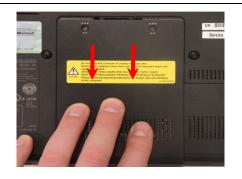
**Step 4.** Slide the Hard Drive Door away from the unit, and lift to remove.
