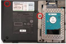
**Step 6.** Using the enclosed magnetic screwdriver, remove the (2) screws securing the ODD Bay.
