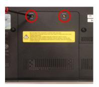
Step 20. Re-install the two (2) Hard Drive Door Screws to secure the Door
