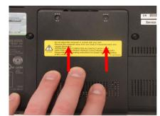
**Step 19.** Re-attach the Hard Drive Door by sliding it towards the unit.
