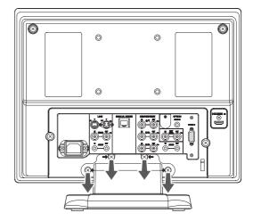
**2** Attach the unit to the rack using the mounting bracket.
