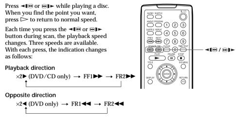
The  $\times 2 \blacktriangleright / \times 2 \blacktriangleleft$  playback speed is about twice the normal speed. The FF2 $\blacktriangleright \blacktriangleright / FR2 \blacktriangleleft \blacktriangleleft$  playback speed is faster than FF1 $\blacktriangleright \blacktriangleright / FR1 \blacktriangleleft \blacktriangleleft$ .
