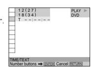
Input the time code using the number buttons, then press ENTER. The player starts playback at the selected time code. To cancel the number, press CLEAR before pressing ENTER.
