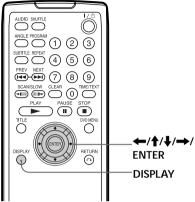
When the player is in stop mode, press DISPLAY and select "SETUP" using **↑**/**↓**.
