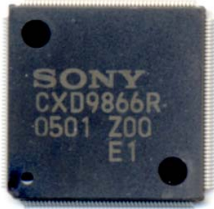
The mathematical algorithms of Sony's Pixel-by-Pixel Active I/P conversion have been committed to silicon in this Large Scale Integrated circuit (LSI), the Sony CXD9866R.
