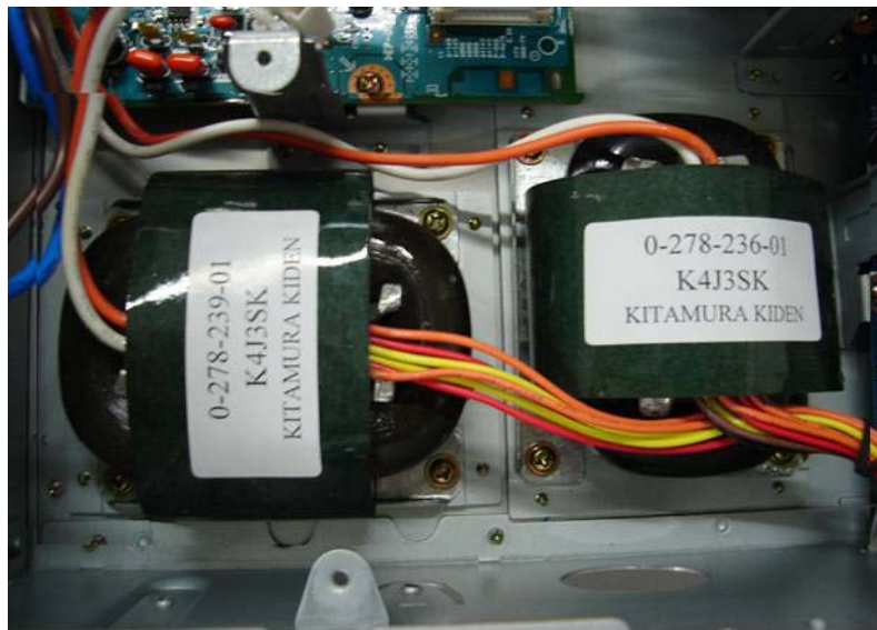
The two power transformers have round cores with cylindrical cross sections. This enables far more consistent transformer windings—for far less radiated hum.
