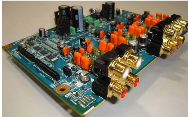
A separate printed circuit board for analog audio employs six separate, identical circuits to handle the 5.1 channels of output.
