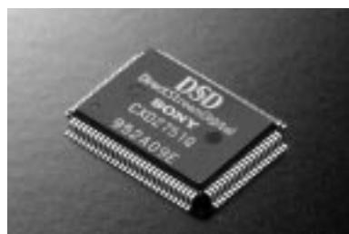
Photo 3: The heart to SACD reproduction, Sony's DSD decoding LSI.
