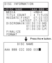
You can change the disc name on the above screen. However, you cannot edit the disc name on this unit. The RM-P110 (not supplied) is required. You can edit the disc name using the RM-P110 (not supplied) connected to the RS-232C connector. For detailed information on the RM-P110, see "To use an RM-P110 (not supplied) as a keyboard for editing/adding title name and information" on page 29.
