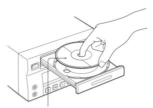
With the recording/playback surface facing down
