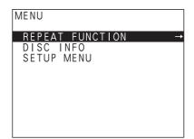
3 Select "REPEAT FUNCTION" by pressing the ♠ or ♠ button, and press the ♠ button with "REPEAT FUNCTION" highlighted.
