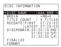
4 Press the ★ or ★ button to select "FINALIZE" and press the ★ button with "FINALIZE" highlighted.
