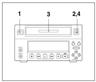
**1** Press the 1 (power) switch to turn the power on.
