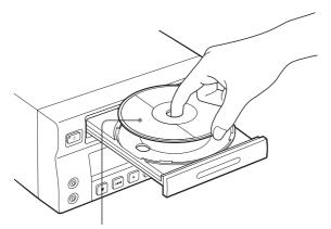
With the recording/playback surface facing down
