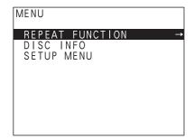
Select "SETUP MENU" by pressing the ♠ or ♥ button and press the → button with "SETUP MENU" highlighted.
