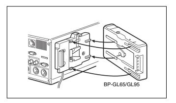
4 Slide the BP-GL65/GL95 as shown below so that the connectors on the BP-GL65/GL95 and the BKP-L551 are connected.
