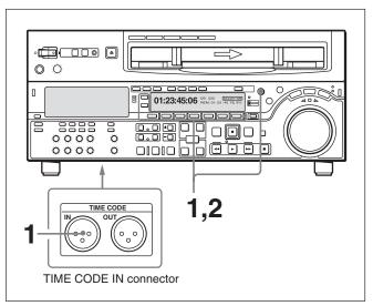
• When synchronizing to an external time code output (LTC):
