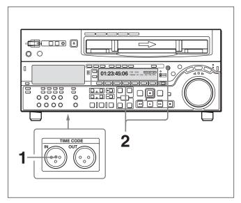
**1** Connect the time code output of the external time code generator to the TIME CODE IN connector.
