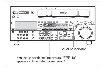
If this happens, the drum and capstan motors stop and the cassette is automatically ejected. Then, the durm starts to rotate again to dry its surface. In this state, the unit is not operable. When the moisture has evaporated, the error message disappears and the ALARM indicator goes off.
