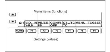
In the figure above, Y-R,B (analog component signals) is selected as the setting for VID.IN, the menu item for button F1. This manual refers to this as "F1 (VID.IN) in function menu HOME page is set to Y-R,B."
