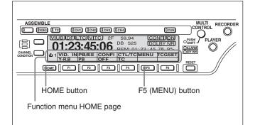
With the function menu HOME page showing in the menu display, press the F5 (MENU) button. The currently selected setup menu item is displayed in the menu display, with the menu item number flashing.
