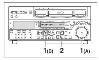
1 (A) Hold down the PLAY button, and turn the search dial in the desired direction to adjust the playback speed.
